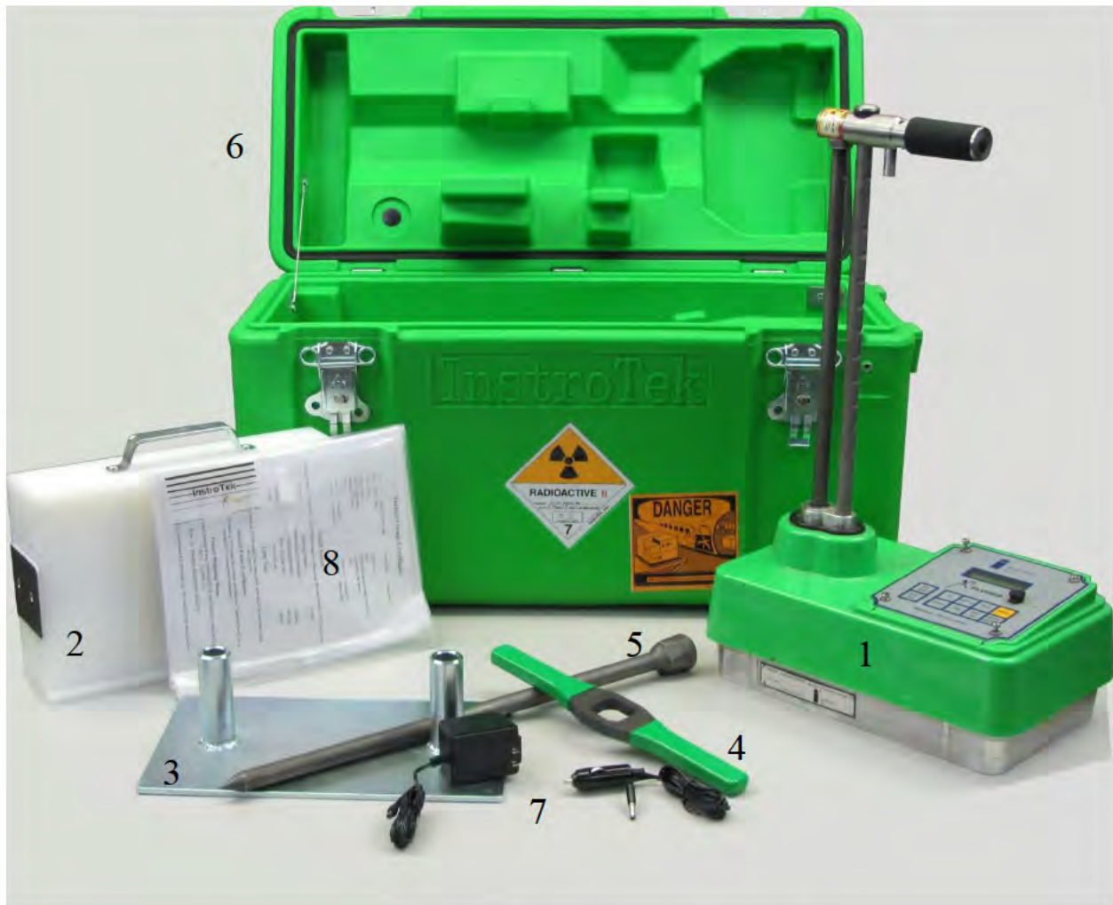
Fig 1.1 Xplorer Nuclear Gauge & Accessories
