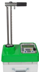
Fig 2.1 Reference Standard Count Position
