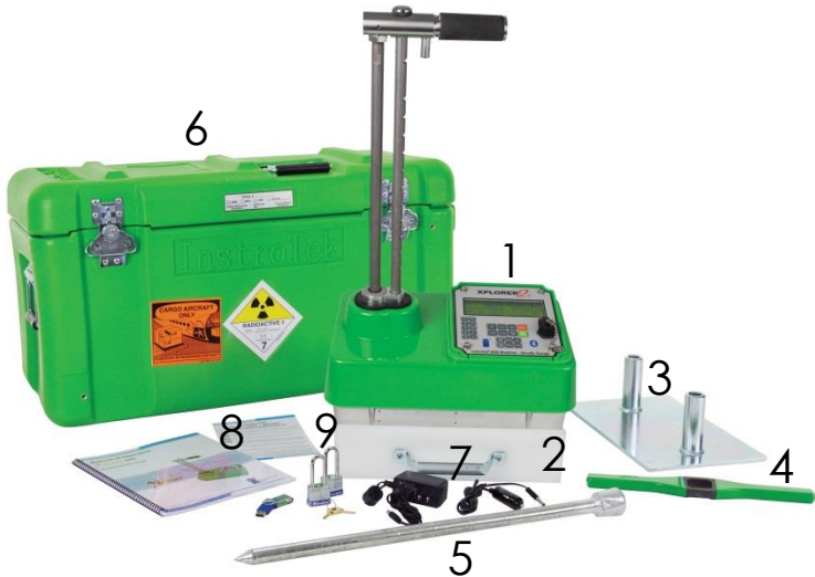
Fig 1.1 Xplorer 2 Nuclear Gauge & Accessories
