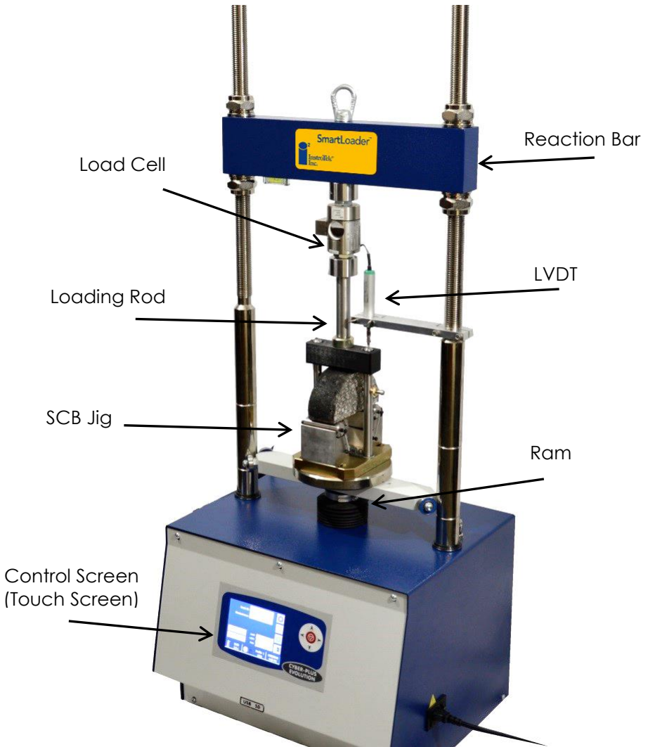
Fig 1. SmartLoader™ Load Frame with SCB Jig
