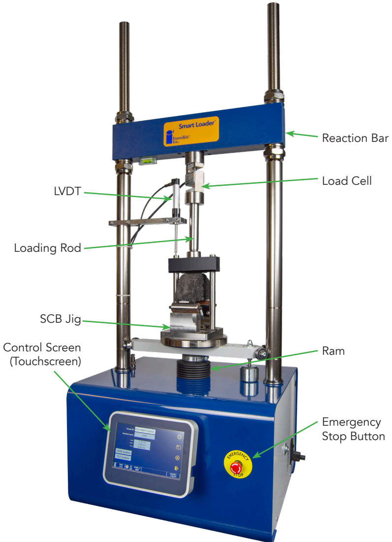
Fig 1. SmartLoader™ Load Frame with SCB Jig
