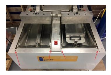
2. Remove the 2 screws securing the tray front.
