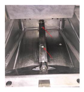
4. Remove the 2 bolts securing the anchor bar.
