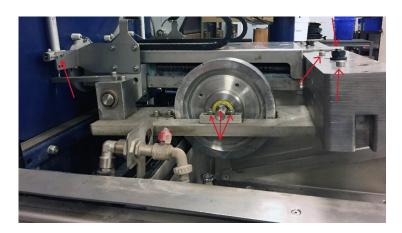
2. Check if the bolts in the picture above are loose. These bolts keep the loading arms level. Also, check that the (3) set screws (red arrows) that hold the arm onto the screw drive are tight.
