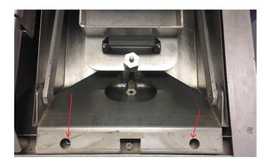
3. Remove the 2 bolts securing the tray bar.
