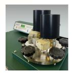
**InstroTek's MiST 2,** the best asphalt moisture sensitivity conditioning device, upgraded with an ultra-quiet pressure system and a small footprint to fit inside any size asphalt lab. MiST 2 test results can determine both the adhesive and cohesive properties of asphalt mixtures to help alleviate moisture issues in the field. The New & Upgraded MiST 2 is quieter, more compact and user-friendly with advanced features to make the system operate more efficiently.
