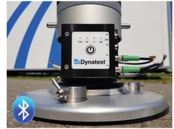
*Integrated Bluetooth® module provides a stable connection*
