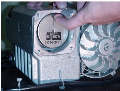
Figure 4: Remove the machine screw holding the filter spring assembly in place.
