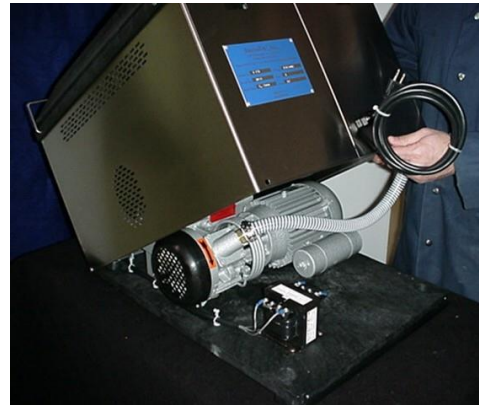
Figure 2: Remove the filler plates and sample from inside the vacuum chamber. Cushion the front of unit with a pad and lift up and forward.
