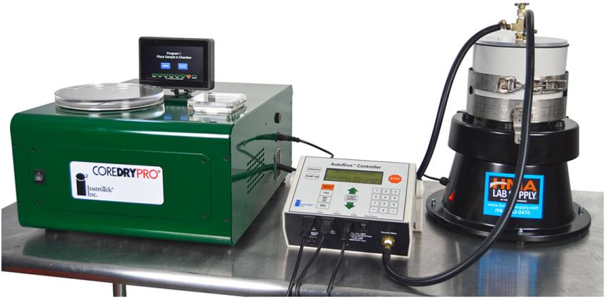
CoreDry set up with AutoRice, pycnometer, and shaker
