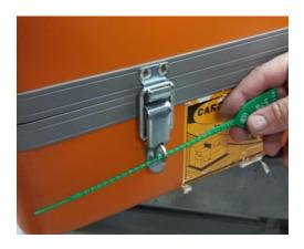
8. Secure the wire tie or lock as shown above. You must make sure that the wire tie is of sufficient size that it will not slip through the slot in the latch hasp allowing the case to be opened.
