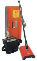
The gauge is part of the Type A Package. The Am241:Be is permanently affixed to inside the gauge.
