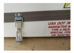
8. Secure the wire tie or lock as shown above. You must make sure that the wire tie is of sufficient size that it will not slip through the slot in the latch hasp allowing the case to be opened.
