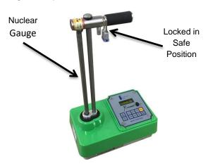
The gauge is part of the Type A Package. The Cs137 is permanently affixed inside the source rod and the Am241:Be is permanently affixed to inside the gauge. The Cs137 source rod locked in Safe position is the start of the packing system.
