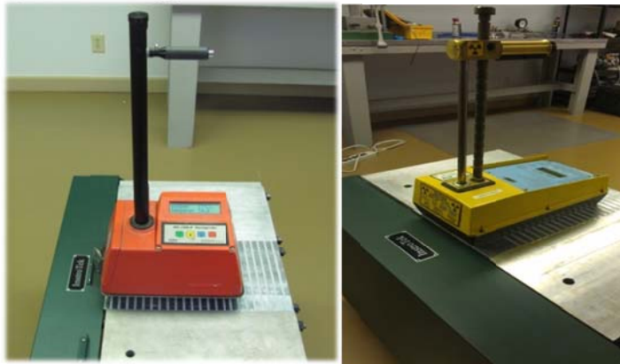
The gauge is placed at the top edge of the block.
