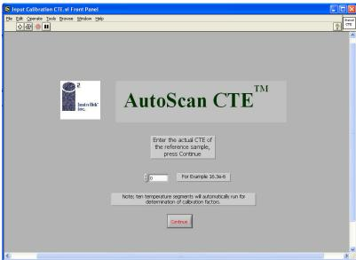
Enter the CTE of your calibration reference standard. For example, for a CTE of  $10.0 \times 10^{-6}$ , enter 10.0e-6.
