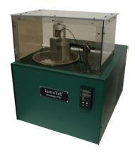
After the LVDT has been adjusted, place the cover on top of the device to protect sample from room ventilation.
