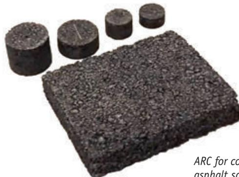
ARC for compacting repeatable asphalt samples
