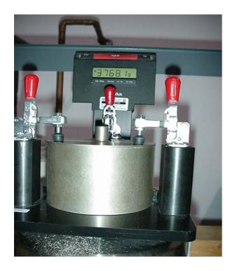
Place the fixture and the container on scales. Measure and record the weight
