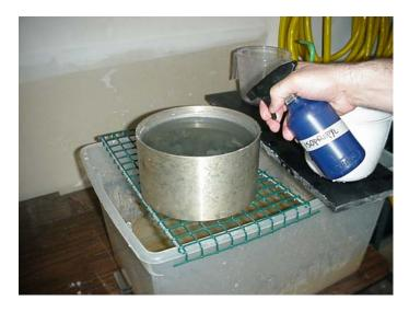
Spray surface of water with alcohol to get rid of any foam or air bubbles on surface.
