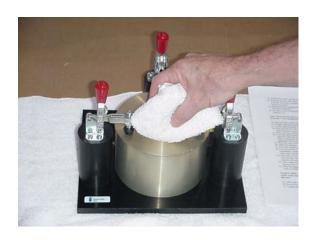
Use a towel to wipe excess water from the 1/8" hole. <u>Do not</u> wipe water from the rim of the container if it seeps between lid and volumeter. Allow this water to remain on fixture.
