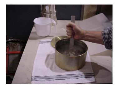
Gently move the aggregate around to remove any trapped air pockets.
