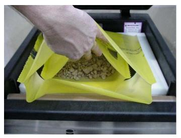
Place the sample (2000 grams for coarse aggregate, 1000 grams for fine aggregate test) into a small bag and place it into the large external bag.
