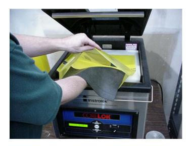
Place the rubber sheet (for coarse aggregates) into the large external bag. Be sure it is centered and pushed all the way to the back of the external bag.
