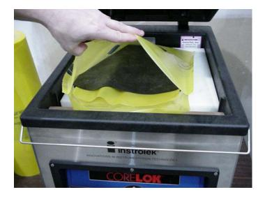
Place the other rubber sheet on top and to the back of the small internal bag. Make sure the two protection sheets completely sandwich the small internal bag and sample. Also it is important that the rubber sheets don't restrict the opening of the small bag.
