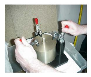
Use the three clamps to clamp the lid down. Be sure 1/8-inch hole faces toward the front.
