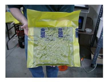
The rubber sheets should completely cover the aggregate.
