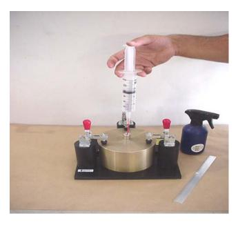
Using the syringe, gently fill the container with water. Place the syringe tip under water level in the volumeter. Don't create air bubbles by injecting too quickly. Add water until water just comes out of small hole. Wipe extra water from around small hole.
