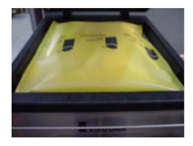
Seal the large external bag with the small bag and protection sheets inside. Be sure only the large bag is exposed to the heat-sealing strip.
