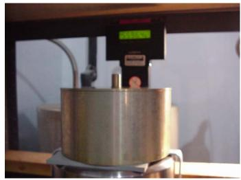
Weigh the volumeter, aggregate, and water. Record the weight.
