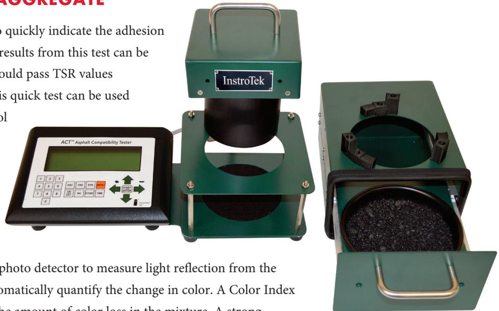
The ACT provides agencies a quick test method to account for routine changes that occur during production and design. This test will ensure that mixture formulation and gradation changes do not negatively affect TSR test results and production of moisture sensitive mixtures.
