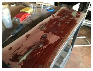
Poor the resin into the gaps. I tend to over fill the gaps as the resin may shrink a little.
