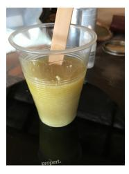
And this is the amount of resin added to it – approximately a 1:3 ratio of powder to resin.
