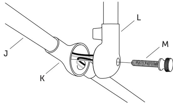
To adjust the Arm angle loosen the Thumb Screw while holding the Arm of the light. Adjust to the desired angle and secure in place by tightening the Thumb Screw.
