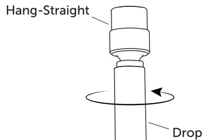
Screw in bulbs fully. If bulb is not fully screwed in, it may appear to sag or be crooked. Though do not over tighten.
