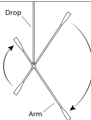
The Hang-Straight hardware allows for the fixture to be rotated and adjusted to hang straight.
