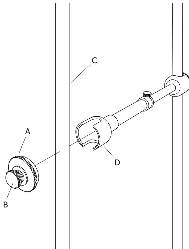
To adjust the length of the Crossbar loosen the Set Screw (E), adjust the telescoping Crossbar to the desired length, and secure the Set Screw again.
