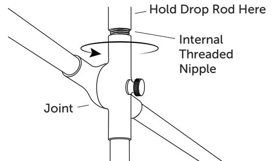
The Hang-Straight hardware allows for the fixture to be rotated and adjusted to hang straight.
