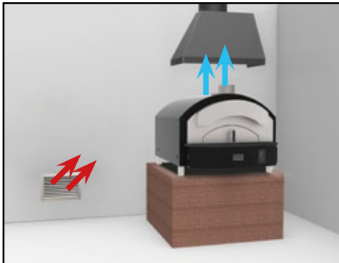
➔ FORCED VENTILATION - 1,72 \text{ m}^3/\text{h} \times \text{kW} ➔ FORCED AERATION - 1,72 \text{ m}^3/\text{h} \times \text{kW}
