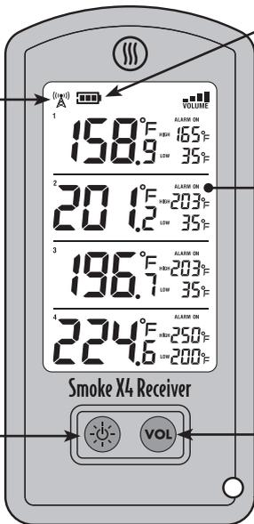
Smoke X4 Receiver display updates every 30 seconds with live temperatures from Smoke X4. It will also show the High/Low Alarm temperature settings and if the alarm is on or off.
