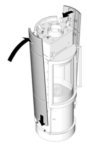
4. Align the threaded studs on the top body brackets into each side's top panel bracket.
