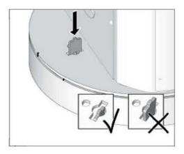
Figure 5: Insert First Rotation Locking Stopper
