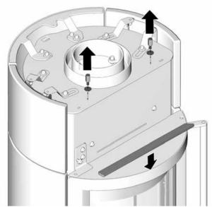
14. Add the top front panel by locating the key slotted brackets to the hardware installed in the front face of the stove body.
