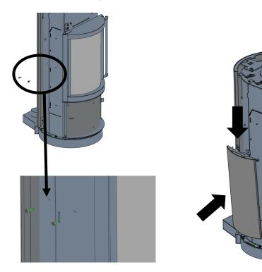
9. Once the lower side stone panel is installed, reinstall the previously removed screws to secure the soapstone panel bracket to the body of the stove. Install the top soapstone panels to the lower panel's top bracket by aligning the panel's bottom holes to the silicone sleeves, and firmly press the stone down onto the bracket.
