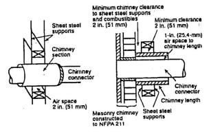
**Figure 3: Chimney Connector Clearances**
