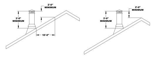
Figure 5: Chimney Height & Roof Clearance Requirements
