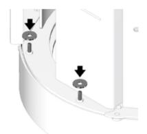
3. For Ceramic Panels: Align each side's bottom holes onto the bottom side studs and push the side firmly down so the threaded studs engage the mounting holes.
