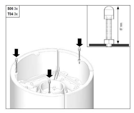
22. For 8171 units with Steel Top Panel: Install the leveling hardware to the indicated levels. Attach the top to the body of the stove and ensure a slight gap between the top and the stove body.
