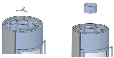
5. Install the provided screws and washers into the threaded holes of the top section of the flue collar to secure the flue collar in place. The screws should hook under the lip of the lower flue collar and allow the flue collar to rotate freely.
