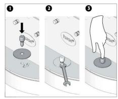
Figure 7: Tighten Mounting Screw
