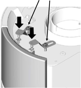
5. Adjust the height of the sides by either adding or removing washers from the bottom threaded studs to line up side panels with the back panels.
