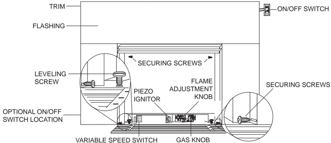
The insert can be equipped with a flashing kit to close off most appliance openings. Mount the flashing inside the unit's outer shell using 4 securing screws. The flashing and trim are available in many finishes to accent any room decor. Objects placed in front of the appliance should be kept a minimum of 48" (1219mm) away from the front face.
