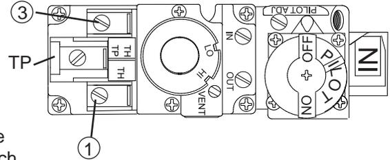
Disconnect the existing wires from terminals 1 and 3 (from the ON/OFF switch) and replace with the leads from the wall switch.
