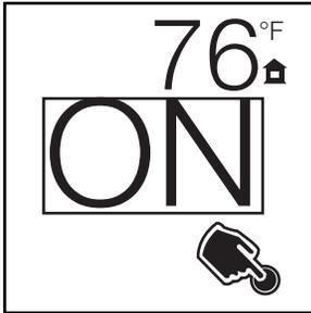
Pressing the AUX function adjustment then toggling the up button "▲" will turn on the LED lights. The initiated light colour is white.
