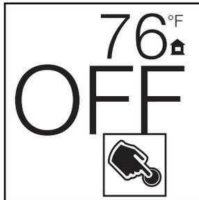
Press the adjustment button down "▼" to turn OFF the LED lights.
