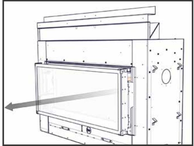
1. To open, release the latches from the GGA-1 using the release tool. Push the release tool against bottom of latch until it disengages from GGA-1. Pull gently on GGA-1 while releasing the latch.
