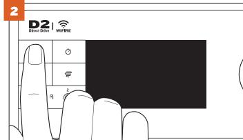
Press any button to turn on the controller.
