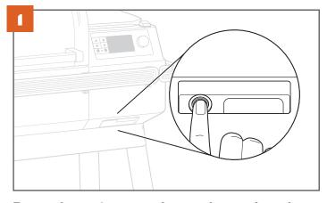
Press the main power button located on the front of the grill to **ON**.
