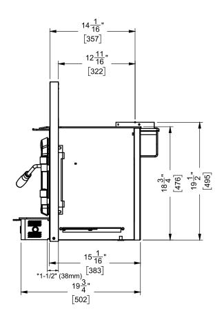
\*Measurement from back of faceplate to fuel door opening
