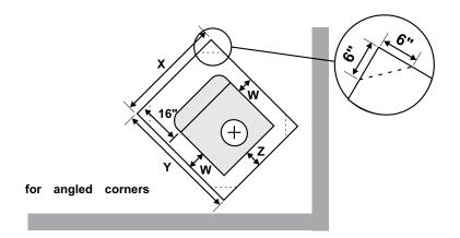
\*\*NOTE: In Canada, floor protection must extend 18" (450mm) to the front and 8" (203mm) to back of the stove.
