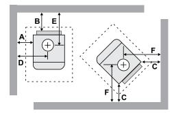
NOTE: This clearance is also required for air space between the appliance and wall/ceiling.
