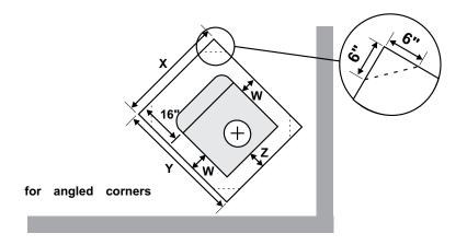
\*\*NOTE: In Canada, floor protection must extend 18" (457mm) to the front and 8" (203mm) to back of the stove.
