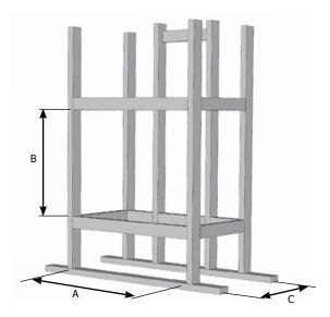
**NOTE:** The appliance must be installed on a flat, solid, continuous surface (e.g. wood, metal, concrete).which must be the full width and depth of appliance.
