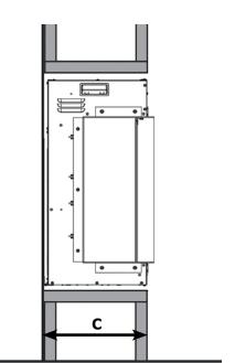
**NOTE:** The appliance must be installed on a flat, solid, continuous surface (e.g. wood, metal, concrete) which must be the full width and depth of appliance.
