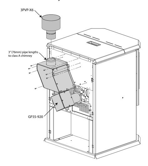
\*In order to achieve the maximum rated efficiency of 75% HHV purchase of a top vent adaptor kit (GF55-920) is required. Use the sheet metal screws provided to attach the kit to the rear of the unit as shown. Please see kit instruction manual for more detailed installation instructions.
