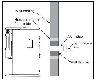
Straight through Wall Installation - Side View
