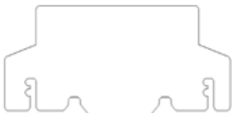
Restrictor plate for Set 1, Set 2 (Part # 761-060F)
