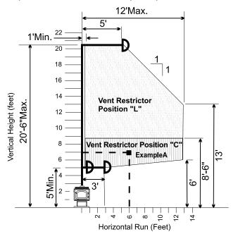
If you are terminating within this shaded area, Vent Restrictor Position "L" (Left) must be used.
