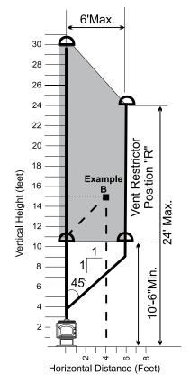
Straight Vertical and Offset to Vertical Terminations use Vent Restrictor Position "R" (Right)
