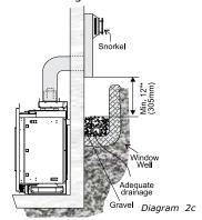
7. Ensure that the pipe clearances to combustible materials are maintained (Diagram 5). Install the termination cap.
