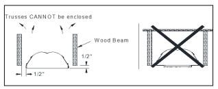
Note: Surfaces between joists or flush with the heater must not exceed 50°C (90°F) above ambient temperature
