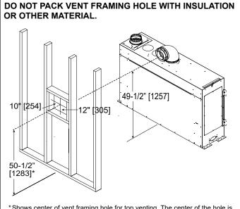
\* Shows center of vent framing hole for top venting. The center of the hole is one 1" (25mm) above the center of the horizontal vent pipe.
