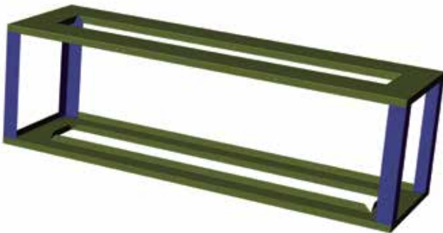
Diagram 3 - Corner supports with top frame
