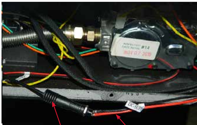
DC supply wire from wiring harness
