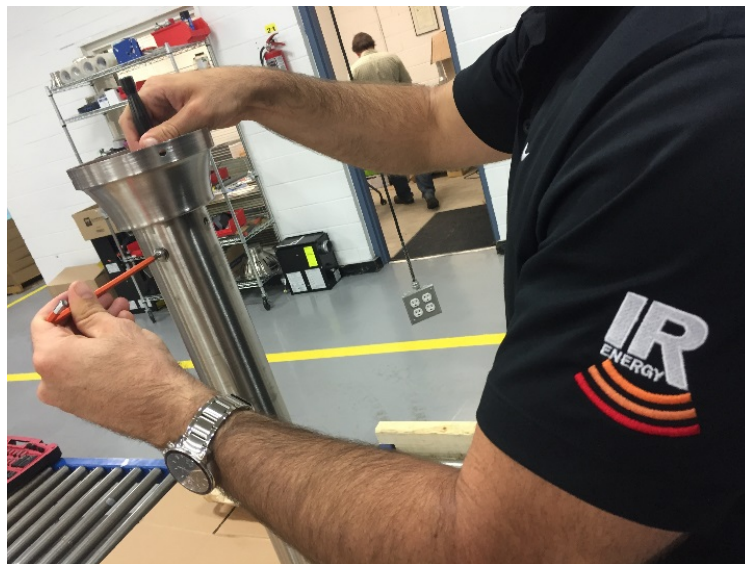
Figure 34: Tighten Pole Neck
