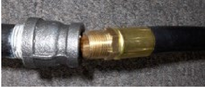
Figure 14: Gas Hose Connections
