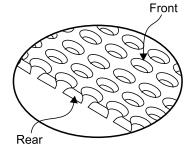
Note: The grill has a front and rear, the holes on the front side have rounded edges and the rear holes have flat edges.
