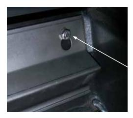
Ensure deflector is seated so bolts are situated at the top of the keyhole before tightening.
