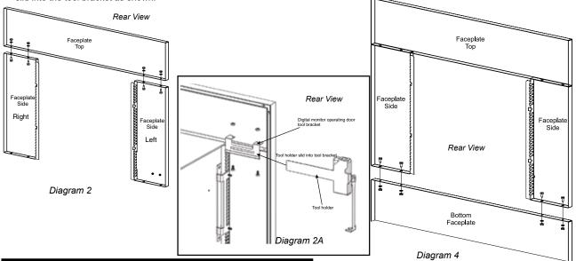
If the insert is going to sit on the hearth proceed to "Faceplate Trim Installation" (step 8) otherwise continue on to "Bottom Faceplate Installation" (step 4).
