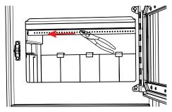
Remove locking clip from the front face of the Catalyst assembly by sliding up and out.
