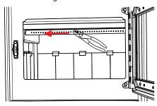
4. Remove left and right baffle brackets (removal of left baffle bracket shown below.
