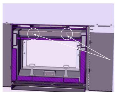
Ensure deflector is seated so bolts are seated at the bottom of the slot before tightening.
