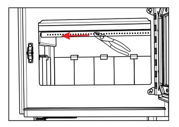
5. To reinstall or replace, first slide left side of tube into hole on left side air channel. Align tab on right side air channel with notch on right hand end of air tube. Firmly grip center of air tube with vise grips, use hammer to tap vise grips from left to right until the tube bottoms out into the air channel on right.
