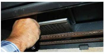
9. Loosen bolts on catalyst retainer then, slide the catalyst retainer to the right to remove.
