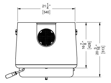
6" (152mm) Diameter STANDARD FLUE ADAPTOR
