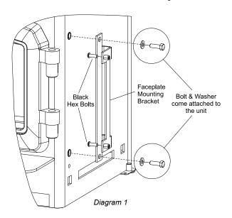
Assemble the faceplate sides and top using the 1/4" x 1/2" long hex bolts, lock washers, and nuts provided. Do not tighten. See Diagram
