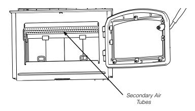
Grasp secondary air tube firmly with vise grips, using a hammer tap vise grips from right to left until air tube is released from grip. Remove.
