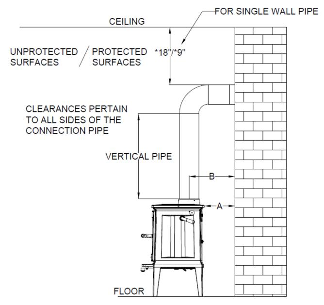
**Figure 5 Chimney Connector Clearances**
