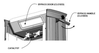
Figure 12 – Bypass Closed
