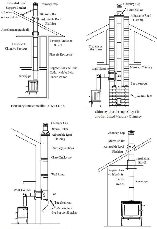
Chimney through outer wall with enclosed chase.
