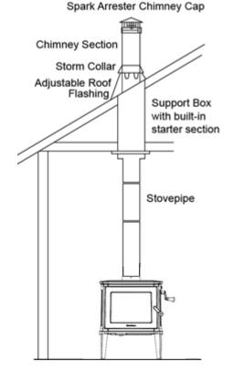
Mobile home installation. One story house installation with attic. Chimney is supported by Ceiling.
