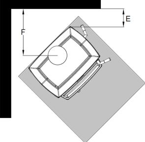
Figure 4 – Clearance to Combustibles
