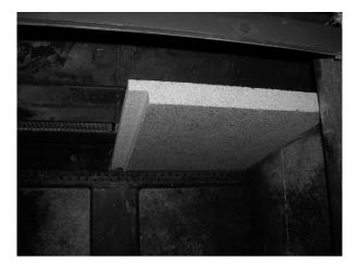
5. Inspect the catalysts for visible damage or fly
