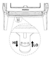
Figure 15 – Air Control Position
