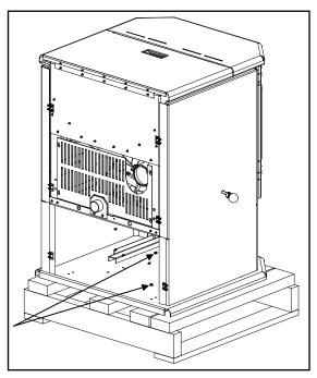
Figure 1: Removing GF55 From Pallet.
