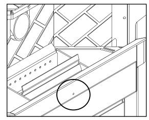
Figure 41: Hole for Pressure test with Magnehelic Gauge
