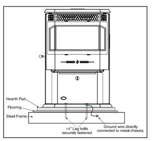
Figure 6: Mobile Home Install Mounting
