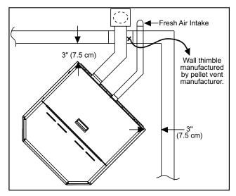
Figure 10: Corner Installation
