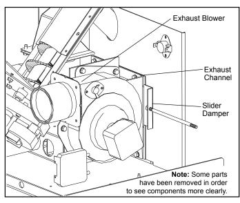
Figure 39: Slider / Damper
