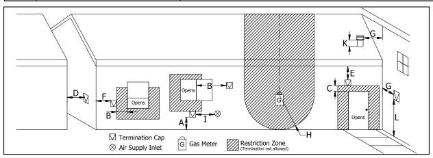
Figure 7: Allowable exterior vent termination locations
