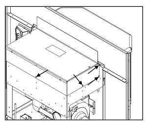
Figure 25: Hopper Extension Screw Placement
