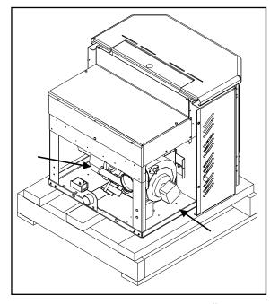
Figure 2: Removing GFI55 From Pallet.
