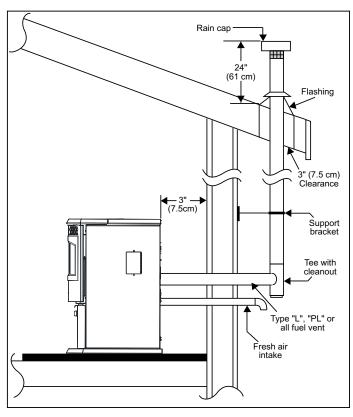
Figure 16: Outside Vertical Installation
