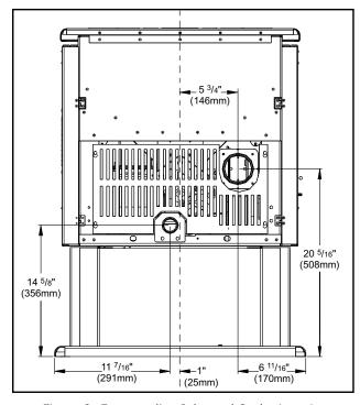
Figure 8: Freestanding Inlet and Outlet Location
