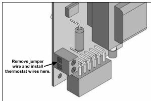
Figure 38: Thermostat wire placement
