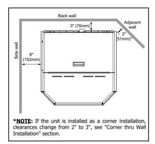
Figure 4: Minimum Clearances to Combustibles
