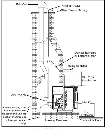
Figure 28: Installation of Fireplace Insert
