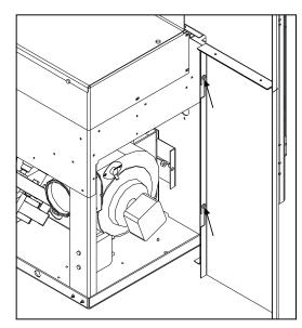
Figure 33: Installed Surround Panel
