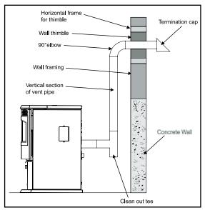
Figure 14: Vertical rise with Horizontal Termination
