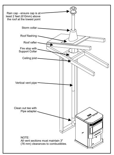
Figure 15: Inside Vertical Installation
