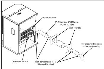
Figure 11: Straight through wall Installation
