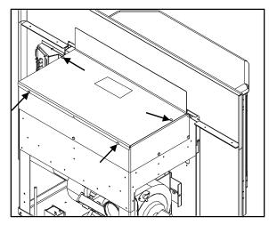
Figure 24: Hopper Cover Screw Placement
