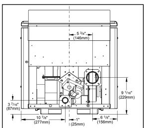
Figure 26: Insert Inlet and Outlet Location
