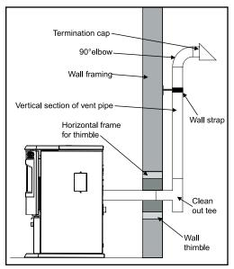
Figure 13: Through Wall with Horizontal Termination
