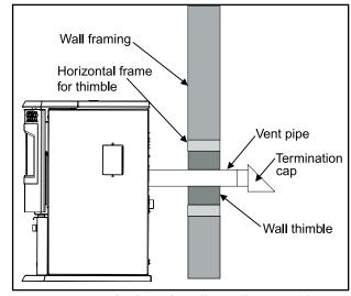
Figure 12: Straight through Wall Installation - Side View
