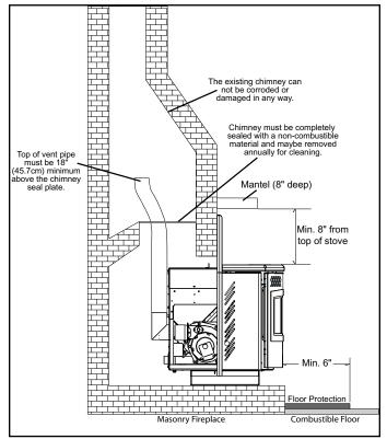
Figure 29: Masonry fireplace positive flue installation
