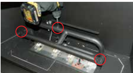
Diagram 2: Slide burner assembly to the right—then remove.
