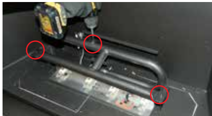
Diagram 2: Slide burner assembly to the right—then remove.
