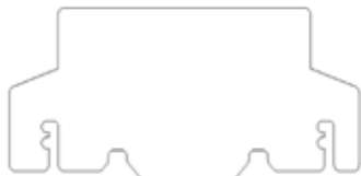
Restrictor plate for Set 1, Set 2 (Part # 761-060F)
