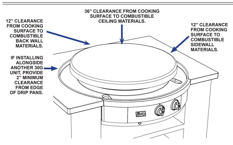
Minimum 3" clearance required under unit venting to 22 sq/in of combustible air. The minimum environmental temperature for safe use of the Evo Affinity 30G should not be below 32°F ( 0° C).
