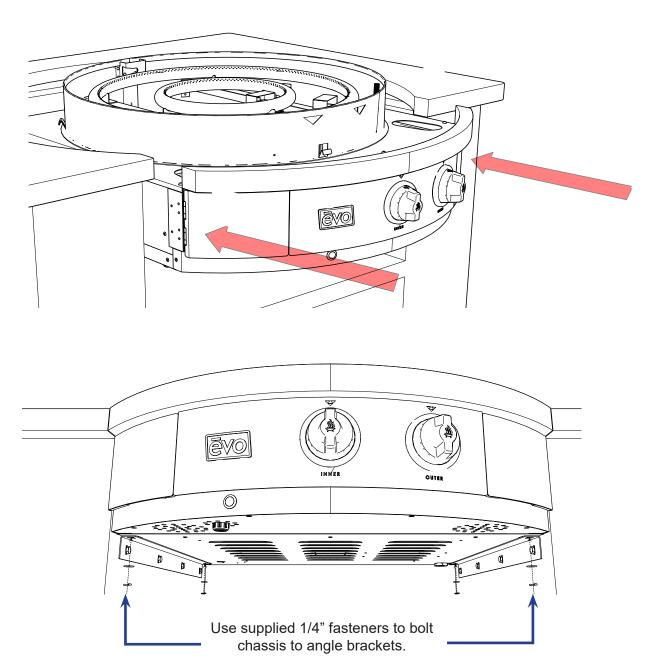
**STEP 4:** Slide the Affinity 30G chassis into the counter top so it rests on top of the installed brackets. Bolt unit to angle brackets using supplied 1/4" x 20 fasteners from underside.
