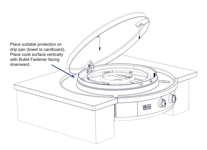
**STEP 8:** Position the cook surface at the rear of the burner chassis by placing the cook surface in the area of the drip pan, separated by a towel or cardboard to prevent damage to the drip pan.
