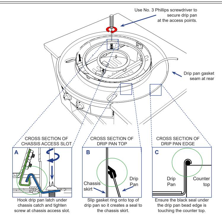
**STEP 6:** Secure drip pan to chassis using access slot (**A**). Rewrap drip pan gasket around top of drip tray and secure (**B**). Ensure seal under drip pan edge is touching counter top(**C**).
