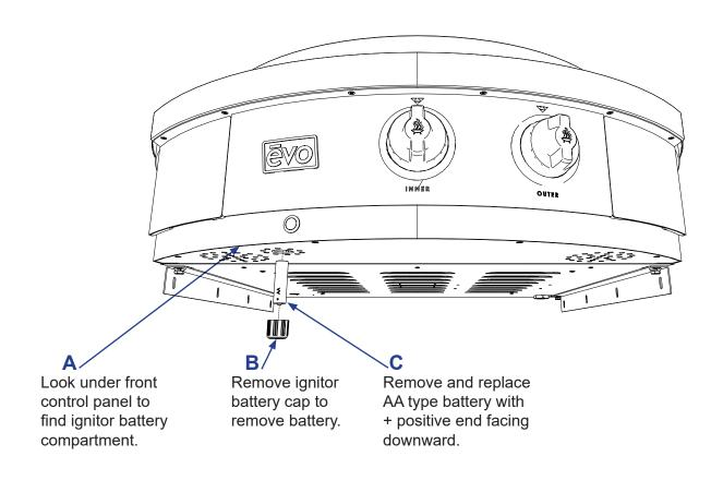
If the ignitor does not work, you may need to replace the battery.
