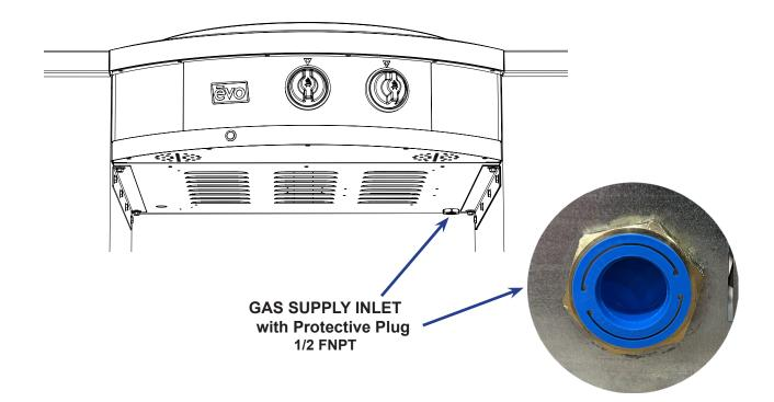
Gas connections for built-in cooking appliances must be a permanent fixed fuel piping system of rigid pipe, semi-rigid tubing, and/or a connector that complies with the Standard for Connectors for Outdoor Gas Appliances and Manufactured Homes, ANSI Z21.75 / CSA 6.27. The maximum length for such gas connections shall be 6 ft (1.82m)
