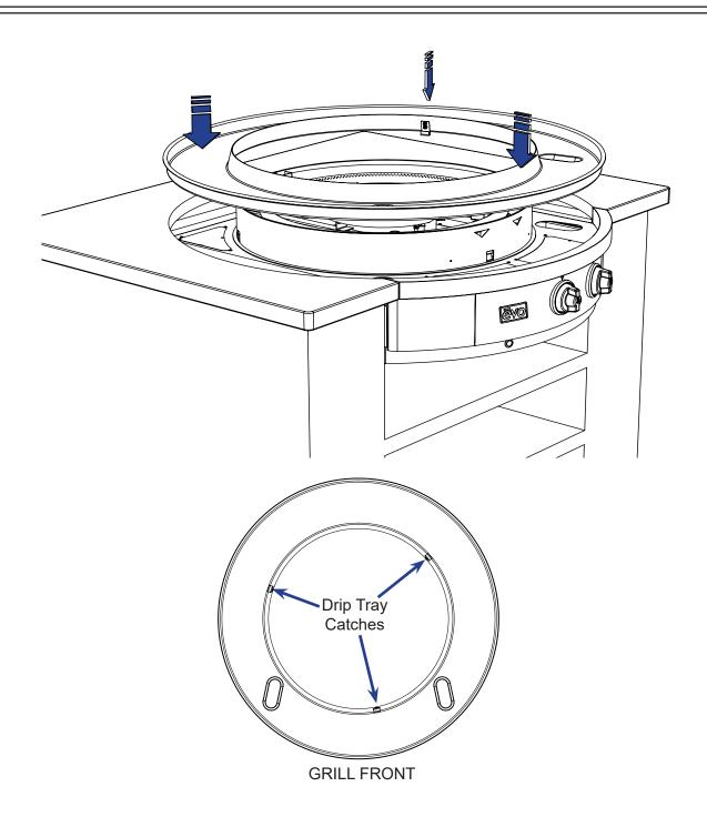
**STEP 5:** Slide drip tray over chassis circular skirt positioning spillover slots to the corresponding slots of the top chassis deck. Notice the drip pan catches showing through the inside cutout locations of the circular chassis skirt. From the inside of the skirt, use each of the three latches to pull the drip pan down into the counter.
