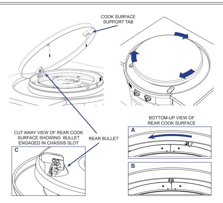
**STEP 9:** Place cook surface over circular skirt with the three support tabs (located under cook surface) resting on the chassis skirt top. Position the rear support tab of the cook surface to the right of the rear seam (rear view) of the chassis skirt (**A**). Then rotate the cook surface clockwise until the support tab is in line with the seam (**B**) and the rear bullet secures in the chassis slot (**C**).
