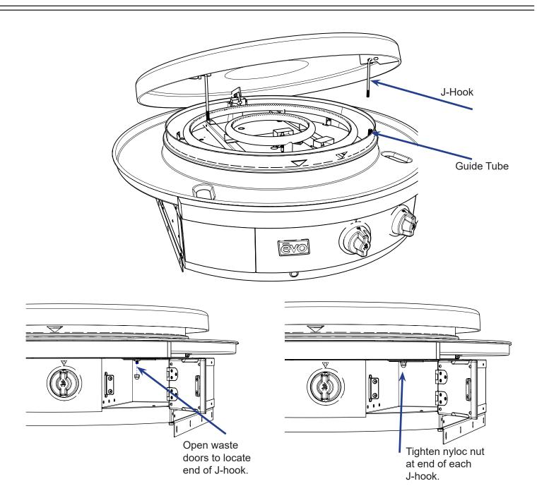
**STEP 10:** Locate two (2) J-hooks attached to underside of cooktop, cut zip ties and remove nyloc nut.
