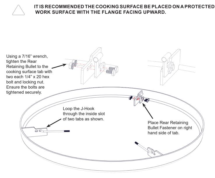
**STEP 7:** Locate Parts Box shipped with your Affinity 30G and the parts bag containing the Rear Retaining Bullet Fastener, two each 1/4" x 20 hex bolt and locking nut, and two each J-Hook. Follow the illustration show on this page, and using a 7/16" wrench tighten the Rear Retaining Bullet to a cook surface tab as shown (Ensure the Rear Retaining Bullet is placed on the right hand side of the tab). Next, loop the J-Hook through the inside slot of each remaining tab.
