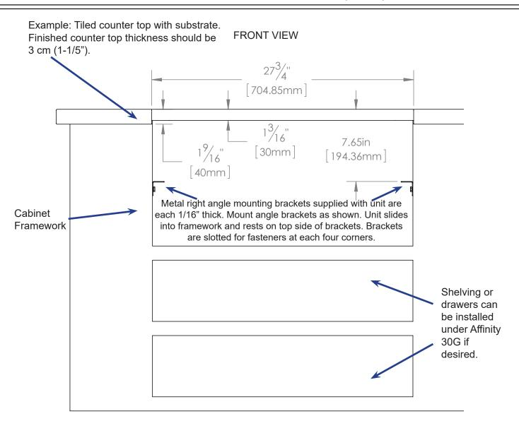
**STEP 3:** Construct a bay for the Evo unit with your chosen cabinet system. Position and fasten the supplied mounting brackets 7.65" below the finished counter top surface.
