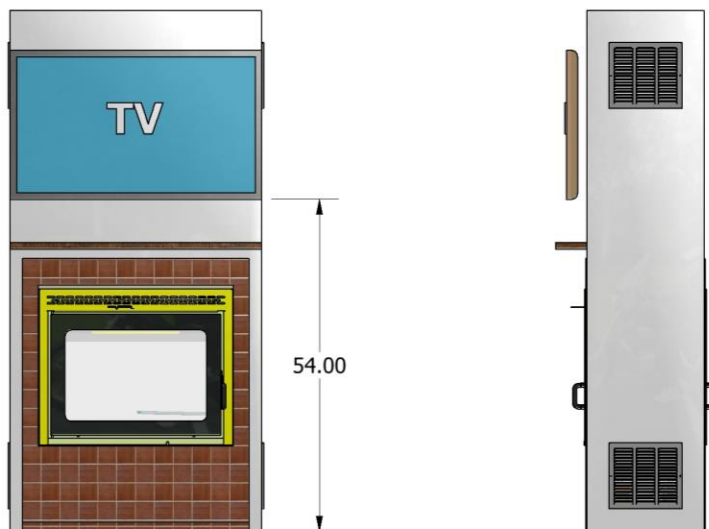
Flat screen television installation A flat screen television can be installed on the face of the fireplace. It is recommended to install a mantle or the header of a mantle to protect the television. The minimum height of the mantle is 44 in. The maximum width of the mantle at 44 in is 5 in.
