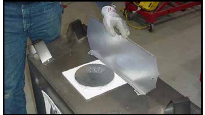
Figure 6.3 Rotate the top heat shield to the vertical position as shown above. The heat shield must remain in the vertical position.
