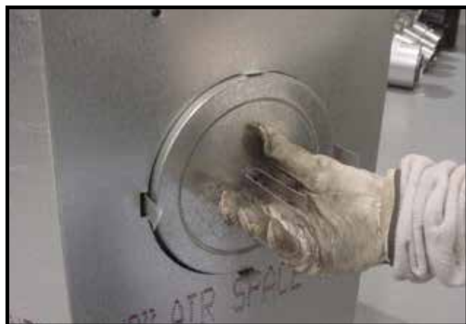
Figure 6.11 Fold the center parts of the retaining band out and use to remove the seal cap.
