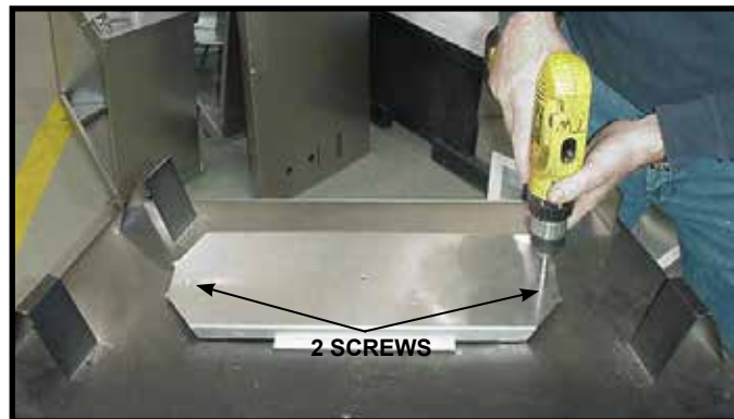
Figure 6.2 For top vent, remove the two screws holding the top heat shield in place.
