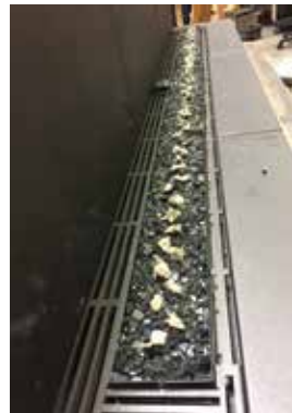
Burner covered with Fireglass and glowing wool
