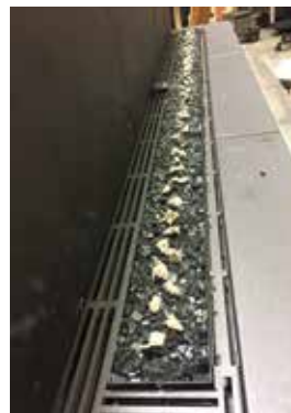
Burner covered with Fireglass and glowing wool
