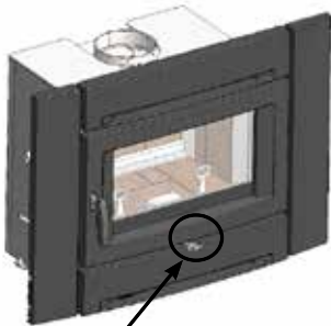
Primary Air Damper Left - Open Right - Closed
