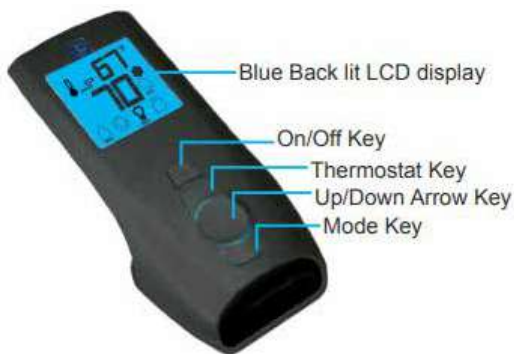
Figure 1: Proflame Transmitter (Part # 911-175)
