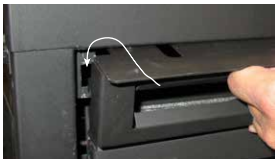
Installation of upper Flush Panel
